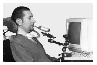
**Integra Mouse**. AbleNet's Integra Mouse enables the user to activate all functions of a computer mouse by mouth. (Source: Photo courtesy of AbleNet Inc.)
