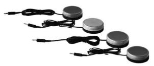
**Access Switch.** A variety of switches, such as these button switches from Prentke Romich, can be used to control a computer. (Source: Photo courtesy of Prentke Romich Co.)
