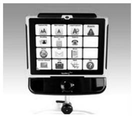
EyeMax. The DynaVox EyeMax system allows augmented communicators to access their Vmax with a simple blink or by dwelling on a desired area of the screen. (Source: Photo courtesy of DynaVox Mayer-Johnson, Pittsburgh, PA [866-DYNAVOX].)
