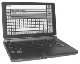
**Freedom LITE.** The Freedom LITE by Words+ is a laptop-based AAC device that works well in workplace settings. (Source: Photo courtesy of Words+.)
