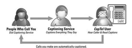
**How the CapTel Works**. A special telephone designed to work with a captioning service displays captions during your telephone calls. (Source: Photo courtesy of Ultratech.)
