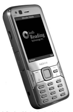
knfbReader Mobile. The knfbReader Mobile from knfb Reading Technology is a portable reading machine that works on a Nokia N82 cell phone. (Source: Photo courtesy of knfb Reading Technology, Inc.)
