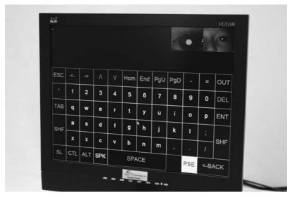
**EyeGaze.** LC Technologies' EyeGaze Edge helps the user control a computer with quick glances and blinking movements. (Source: Photo courtesy of LC Technologies.)
