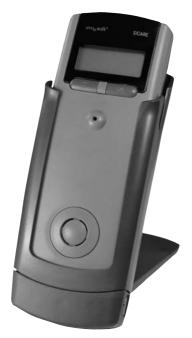
SiCare Standard. The SiCare environmental control unit lets users control numerous appliances and devices by voice alone. (Source: Photo courtesy of AbleNet Inc.)
